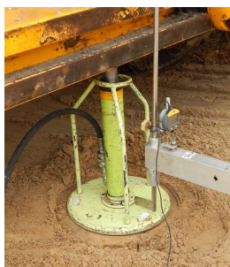
Figure 6 – Stamp warping at soil base tests conducting
